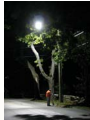
A researcher takes illuminance readings under CMH lighting
